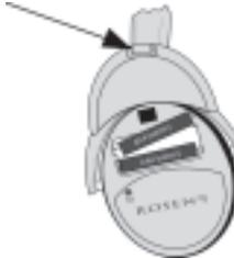
**Step 3** - Remove the batteries and insert the new replacements, noting to insert them correctly.
