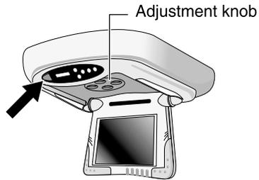
*For 10.4" screens:* Press the release button, as shown. The screen releases slightly and powers on automatically. Manually position it for optimal viewing.
